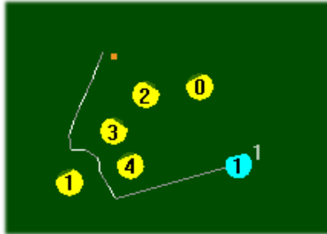
Fig. 15. The robot path generated from RRT path planner.
