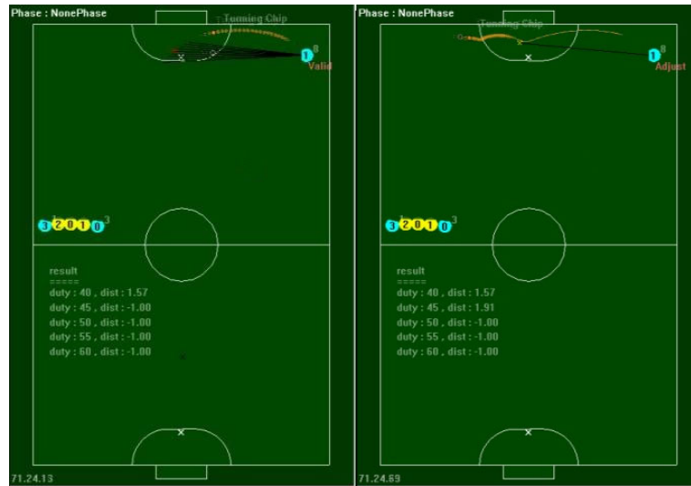
Fig. 21. Snapshots of the chip-kicker calibration process.
