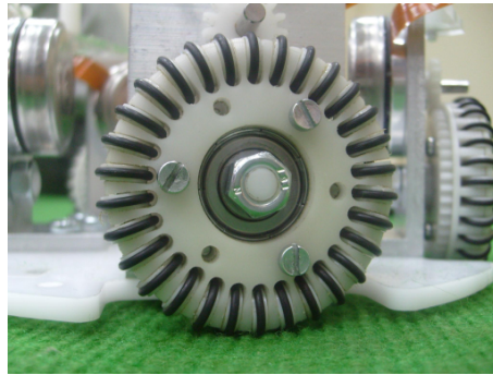
Fig. 2. Locomotion system: omniwheels.
