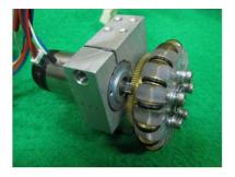
Figure 2. Motor, gear, and wheel assembly.
