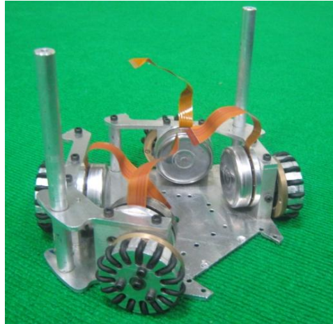
Fig. 3 Robot's chassis with wheels and motors
