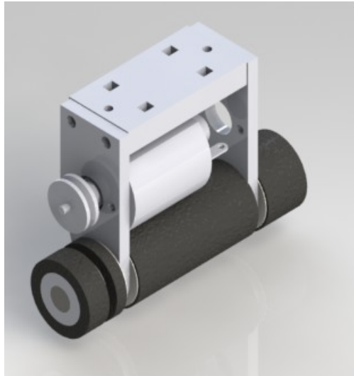
Fig. 4. 2011 dribbler design which had some mechatronic design flaws. A second iteration of this dribbler concept is planned for 2012
