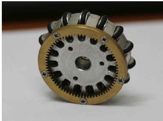
Fig. 6 Inside view of our Omni-Wheel
